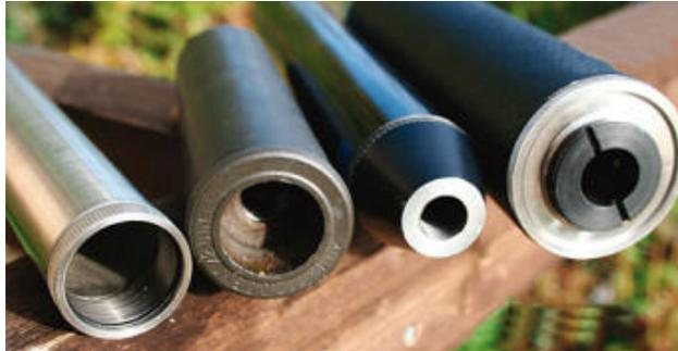
This is the correct term for what most people refer to as a silencer. They attach to the end of the barrel and suppress the muzzle report. They really serve no purpose for target shooting as invariably they rob the rifle of a small amount of power and can also cause a zero shift due to the internal vortexes caused by the pellet moving through a
